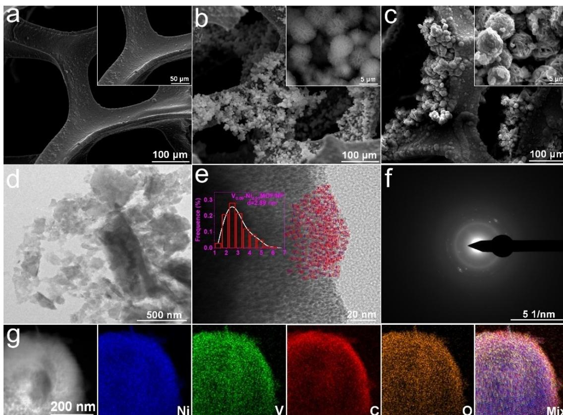
**Figure 2.** SEM images with (inset) high-magnification SEM images of a) bare NF, b) NiV-OH/NF, and c)  $V_{0.09}\text{-Ni}_{0.91}\text{MOF/NF}$ . d) TEM image, e) high-resolution TEM image with (inset) distribution of particle size diameter, f) SAED image, and g) HAADF-STEM image and the corresponding element mappings of  $V_{0.09}\text{-Ni}_{0.91}\text{MOF/NF}$ .
