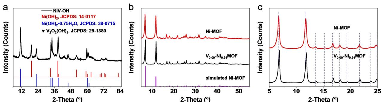
Figure 1. XRD patterns of a) NiV-OH, b) Ni-MOF, V<sub>0.09</sub>-Ni<sub>0.91</sub>MOF plus simulated Ni-MOF, and c) narrow-range XRD of Ni-MOF and V<sub>0.09</sub>-Ni<sub>0.91</sub>MOF.
