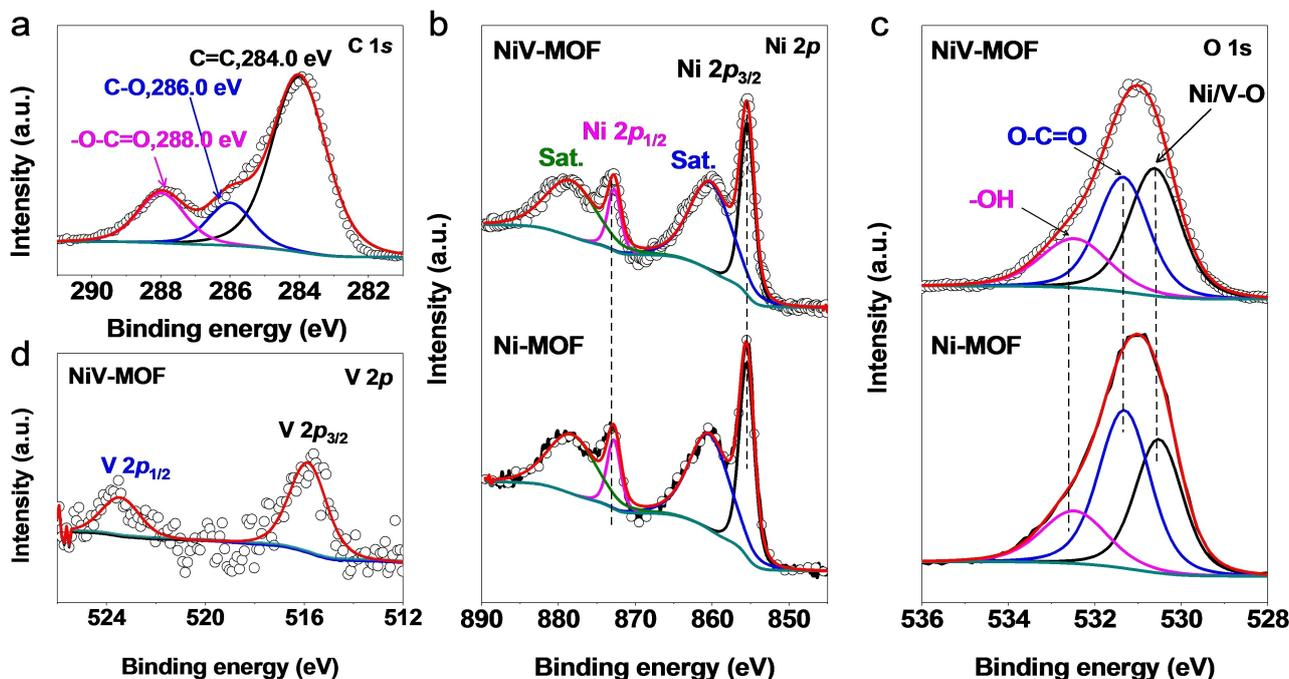
**Figure 4.** XPS spectra of a) C 1s and b) Ni 2p of  $V_{0.09}\text{-Ni}_{0.91}\text{MOF}$  and Ni-MOF, c) O 1s of  $V_{0.09}\text{-Ni}_{0.91}\text{MOF}$  and Ni-MOF, and d) V 2p of  $V_{0.09}\text{-Ni}_{0.91}\text{MOF}$ .
