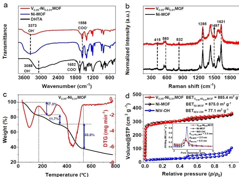
**Figure 3.** a) FTIR spectra of  $V_{0.09}\text{-Ni}_{0.91}\text{MOF}$ , Ni-MOF, and the DHTA ligand. b) Raman spectra of  $V_{0.09}\text{-Ni}_{0.91}\text{MOF}$  and Ni-MOF. c) TGA and DTG analysis of  $V_{0.09}\text{-Ni}_{0.91}\text{MOF}$  in  $N_2$ . d)  $N_2$  adsorption-desorption isotherms with pore size distribution (inset) curves of  $V_{0.09}\text{-Ni}_{0.91}\text{MOF}$ , Ni-MOF and NiV-OH.
