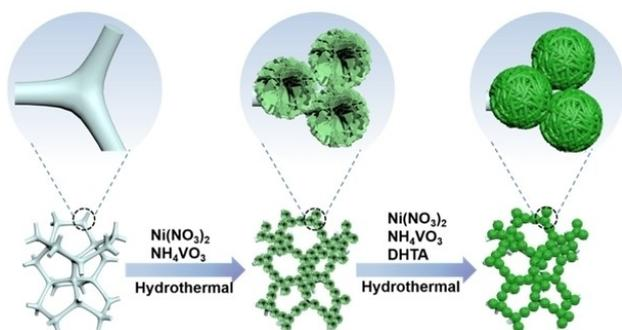
Scheme 1. Schematic illustration of the synthesis of V<sub>0.09</sub>-Ni<sub>0.91</sub>MOF/NF.
