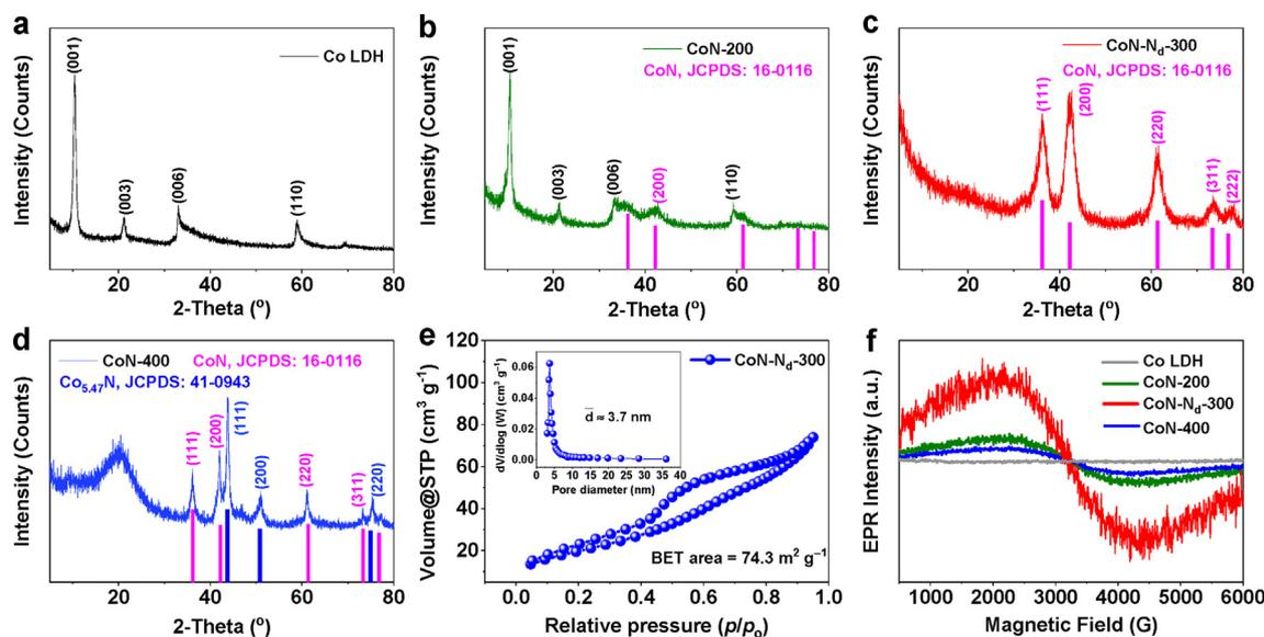
**Fig. 2.** (a-d) XRD of Co LDH, CoN-200, CoN-N<sub>d</sub>-300, and CoN-400. (e) Nitrogen adsorption–desorption isotherms and the BJH pore-size distribution curves (inset) of CoN-N<sub>d</sub>-300. (f) The ESR spectra of CoN-N<sub>d</sub>-300 (peeled off from the CC).
