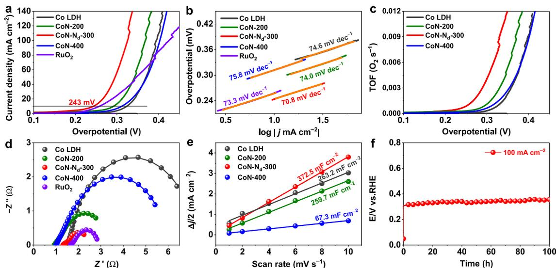
Fig. 5. Electrocatalytic OER performance. (a) LSV polarization curves, (b) corresponding Tafel slopes, (c) potential-dependent TOF curves, (d) electrochemical impedance spectroscopy (EIS), (e) summarized double-layer capacitance ( $C_{dl}$ ) of Co LDH, CoN-200, CoN-N<sub>d</sub>-300, CoN-400, and RuO<sub>2</sub> in 1.0 M KOH. (f) Durability test of CoN-N<sub>d</sub>-300 at 100 mA cm<sup>-2</sup> in 1.0 M KOH.
