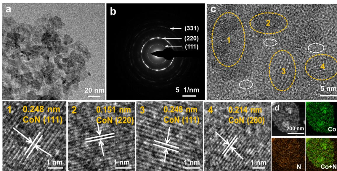
**Fig. 3.** (a) TEM image, (b) SAED and (c) High-Resolution TEM images, and (d) HAADF-STEM image and corresponding elemental mappings of CoN- $N_d$ /CC (color online).
