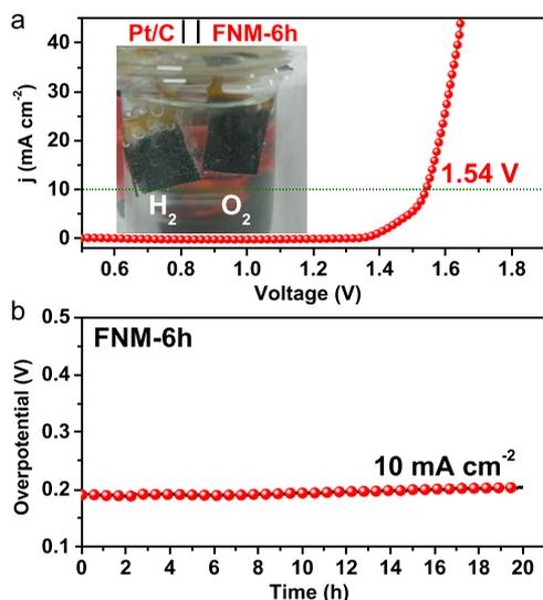
**Figure 5.** (a) Overall water splitting of  $\text{Fe}_{0.38}\text{Ni}_{0.62}$ -MOF and commercial Pt/C on CC surface as anode and cathode electrocatalysts in two-electrode system. (b) Long-term stability test of  $\text{Fe}_{0.38}\text{Ni}_{0.62}$ -MOF/CC catalyst continuously operated at  $10 \text{ mA cm}^{-2}$  for 20 h.
