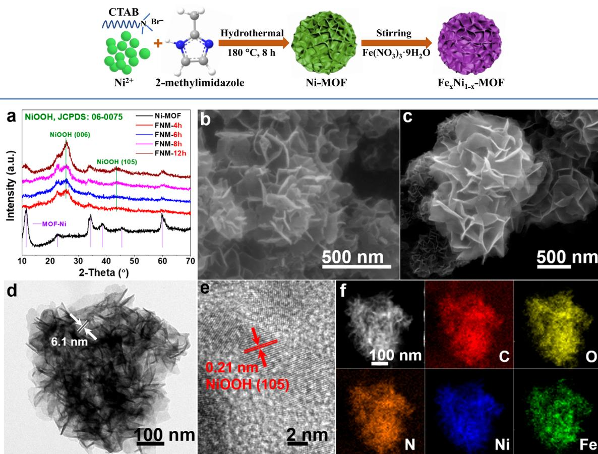
**Figure 1.** (a) XRD patterns of Fe modulated Ni-MOF with different reaction times. SEM images of (b) Ni-MOF and (c)  $\text{Fe}_{0.38}\text{Ni}_{0.62}\text{-MOF}$ . (d) TEM and (e) HRTEM images of  $\text{Fe}_{0.38}\text{Ni}_{0.62}\text{-MOF}$ . (f) HAADF-STEM image of  $\text{Fe}_{0.38}\text{Ni}_{0.62}\text{-MOF}$  and the corresponding elemental mappings of C, O, N, Ni, and Fe.
