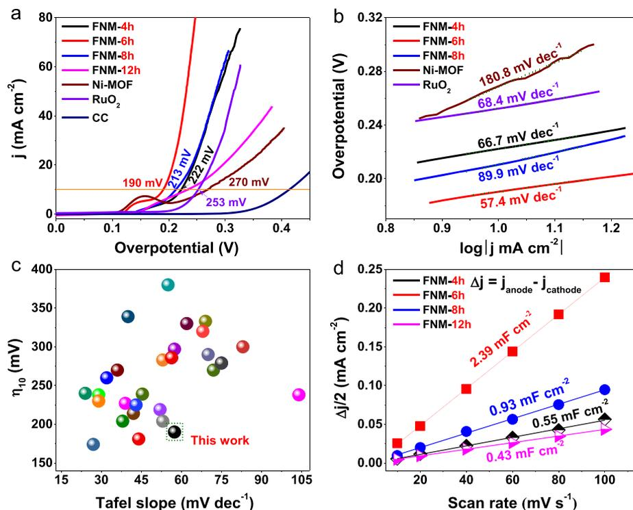
**Figure 4.** OER catalytic performance of different catalysts in 1.0 M KOH. (a) LSV curves with a scan rate of 0.2 mV s<sup>-1</sup>. (b) Tafel slopes calculated from LSV curves. (c) Summarized overpotentials of the recently reported catalysts at 10 mA cm<sup>-2</sup> and the corresponding Tafel slopes (Table S2). (d) Summarized double-layer capacitance ( $C_{dl}$ ) of different catalysts.
